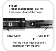
inner of the tracks towards you until it separates completely from the unit. Set track inner with collar attached aside in a safe location.
