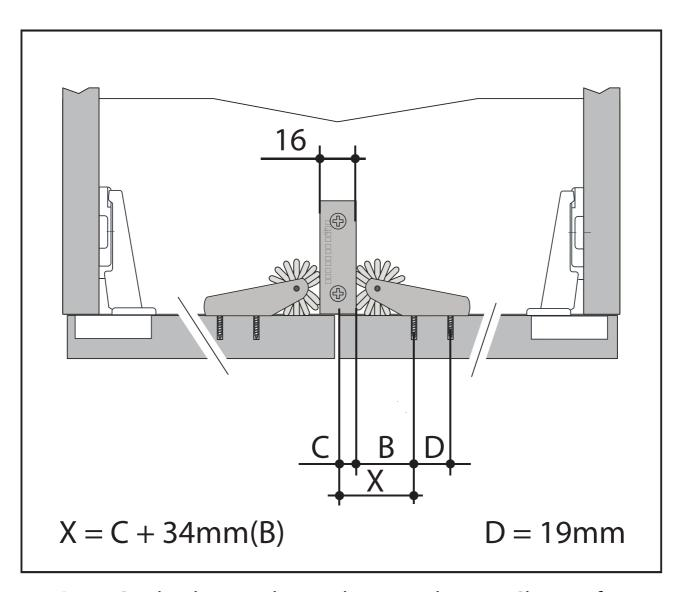
Daisy Catch Inline can be used against the Easy Cleat surface or directly against an end panel
