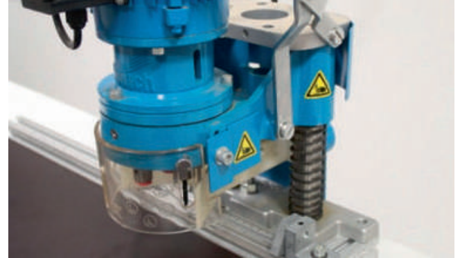
Fig. 4: Sliding guard at drilling spindles
