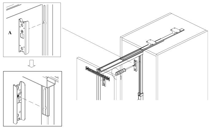
Step 2:Put the plastic clip on bracket, then hold the basket.
