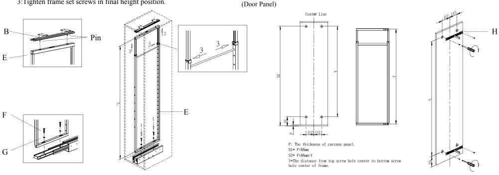
STEP 5: 1.Release middle screw of T-Bar, push together T-Bar to frame tubing, then tighten the middle screw and two screws on T-Bar.
