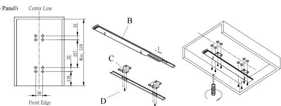
STEP 4:1:Mark center line and screw hole positions on bake of door panel for two T-Bar (H).
