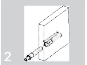
The base provides a flange for positioning on the edge of the furniture. Secure the  $\emptyset 3x12$  screw and then introduce the dampener on the front.
